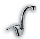
Single lever, pillar type. flow rate restricted to 3.6 ltrs/min G1/2" female connection ends.
